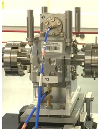
A position cavity installed at STFC Daresbury
