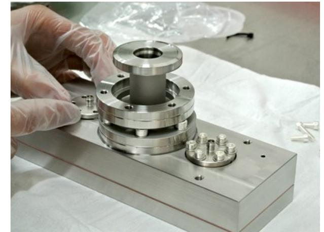
A prototype reference cavity during assembly
